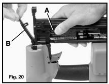
**WARNING:** Disconnect tool from air supply and/or remove battery before removing or reinstalling rubber nose cushion.
